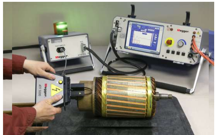
Testing an armature using the ZTX accessory and the ATF5000 commutator probe.
